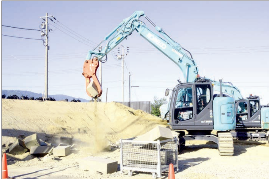
This photo shows a heavy machine being remotely operated during a trial in Kobe, Hyogo Prefecture, in October 2025. PHOTO: KYODO
