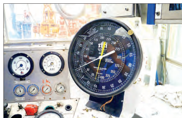
The photo shows an oil rig weight indicator system, a critical piece of industrial instrumentation used on oil and natural gas drilling platforms. PHOTO: PIXABAY
