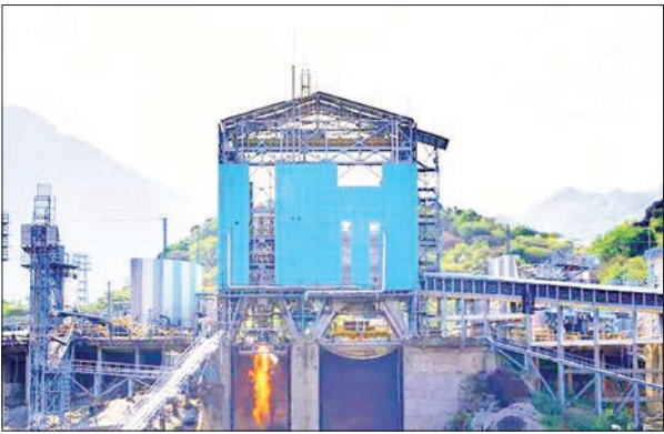
The image shows the flight acceptance hot test of ISRO’s CE20 cryogenic engine at an uprated thrust of 220 kN. PHOTO: ANI
